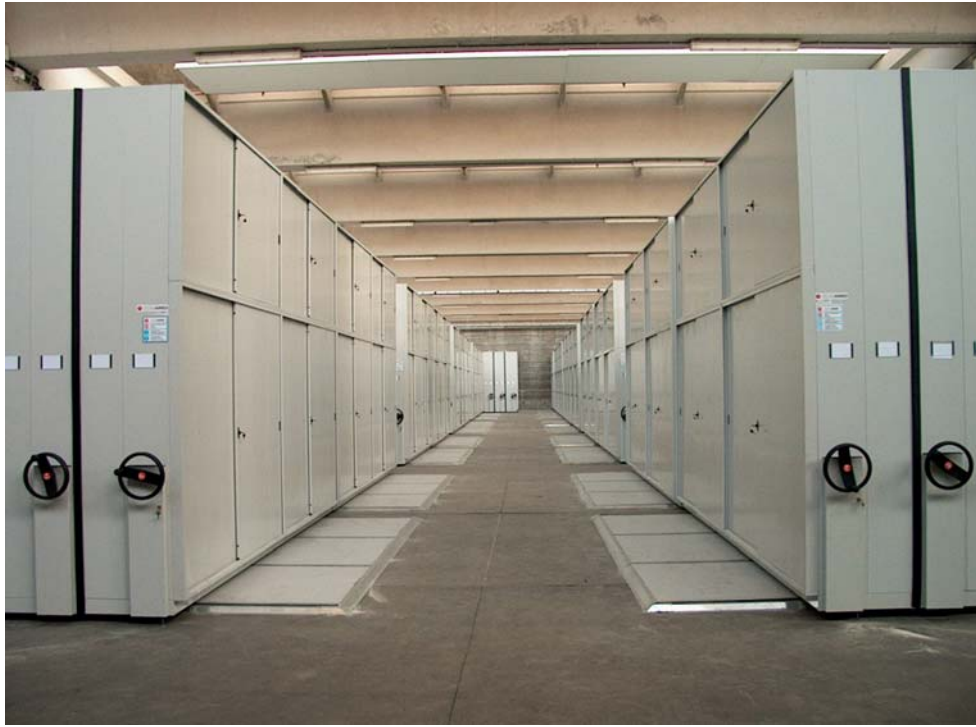
TELECOM ITALIA, COMPANY MAIN ARCHIVE 33.000 linear meters, manual drive
